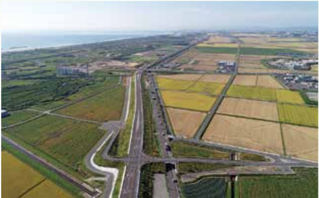
▲ Elevated road, which was developed from recycled tsunami sediment
